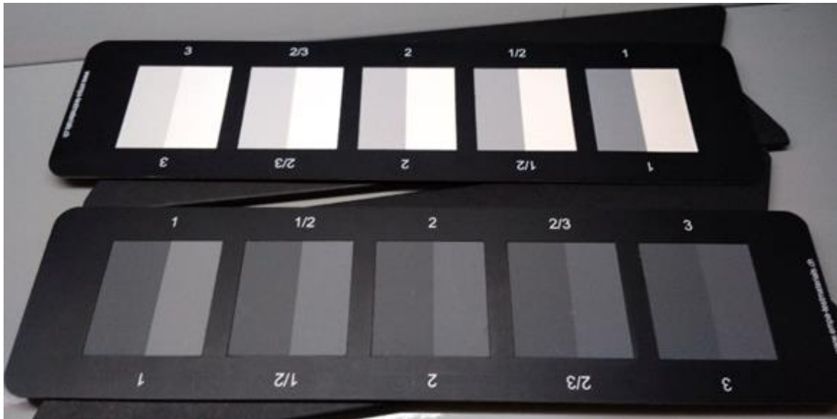
Figure 1: Part of the grayscale (grades 1-3) to assess staining (top) and colour change (bottom)
